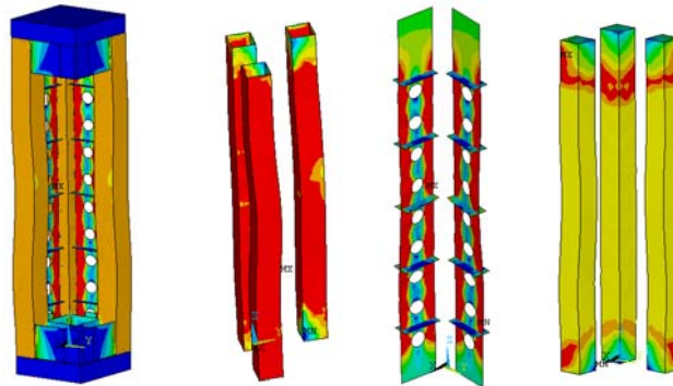
(a) Column (b) Steel tube (c) Connection plates (d) Concrete Figure 16. Strain and Deformation of S-3 (Axial Loading)
