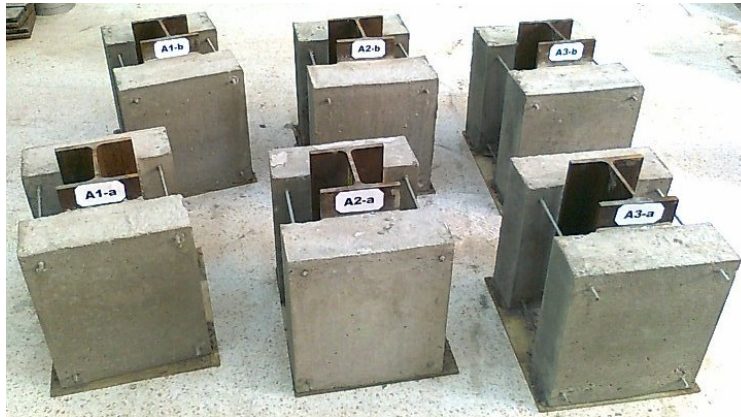
Figure 2. Push-out Specimens of the Series A
