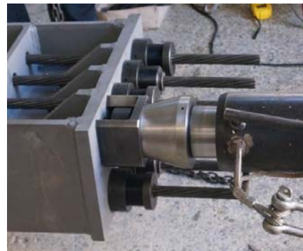
(b) Pretensioning the strands
