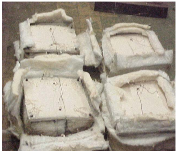
Figure 2. Small scale samples after fire test
