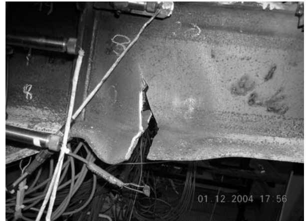
Figure 18. Yielding rupture in the beam at the haunch toe
