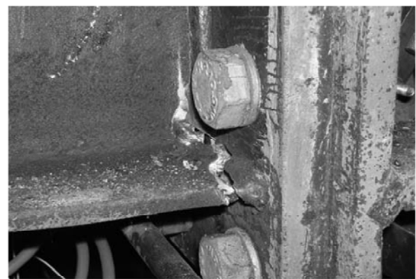
Figure 20. Rupture of welds and fracture of beam web in heat affected zone (HAZ)
