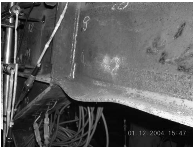
Figure 25-1. Buckling of beam web and beam bottom flange: haunch specimens
