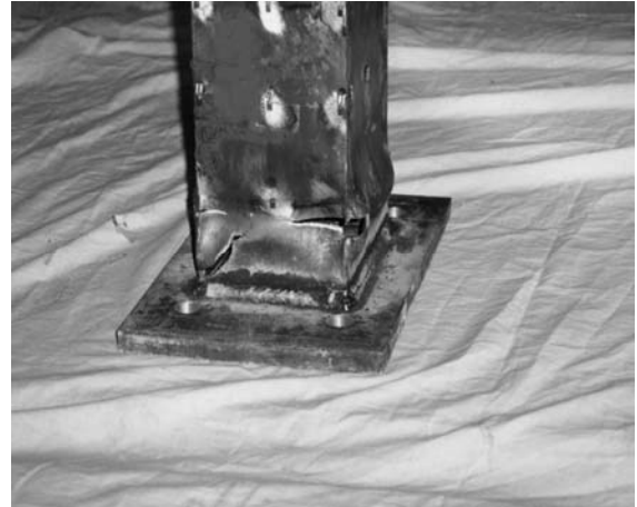
Figure 8. Fracture of member S-5-0
