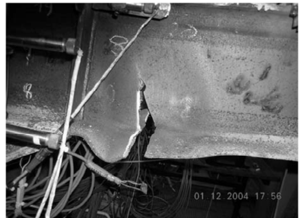
Figure 18. Yielding rupture in the beam at the haunch toe
