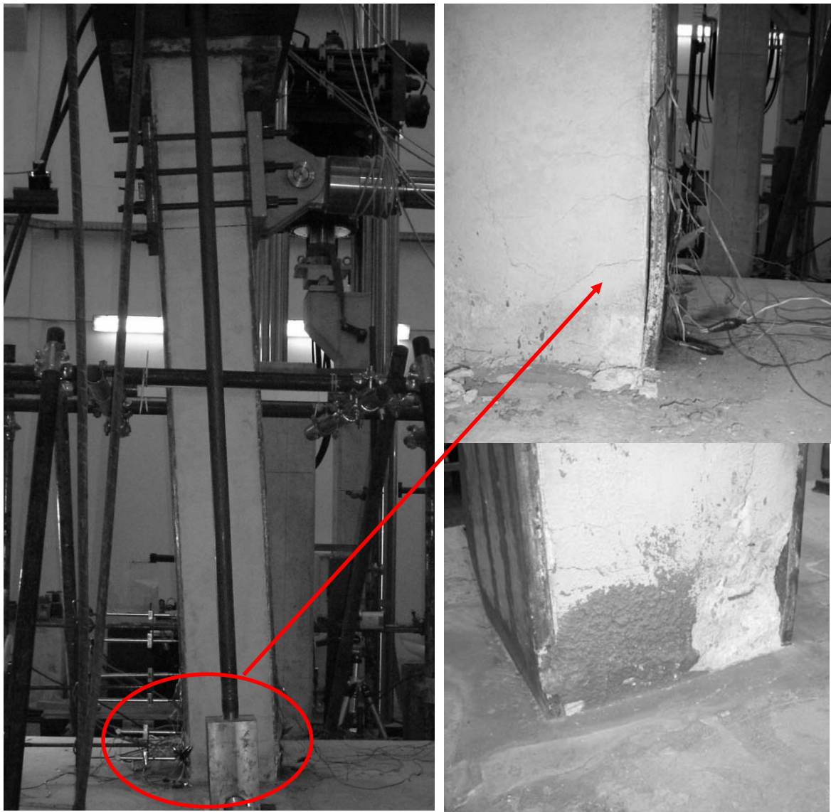
Figure 9. Close-up of the deformations of the specimen HEB260 with N=330\text{kN} .
