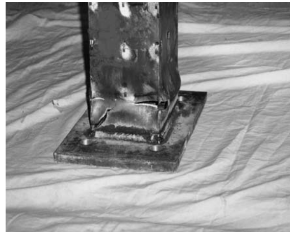
Figure 8. Fracture of member S-5-0
