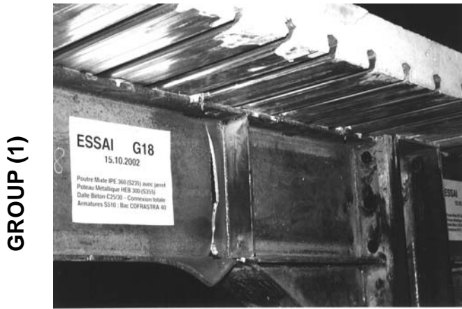
Figure 17. Yielding rupture in the beam at the haunch toe
