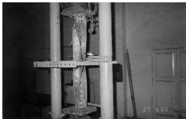
Figure 14. Torsional Buckling of Starred Angle with Bolted End Connection
