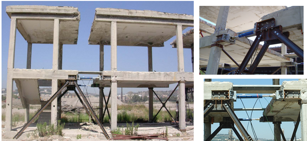
Figure 10. Pushover Test on the Module under Study
