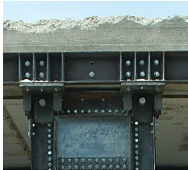
Figure 19. Reaction Steel Frame – RC Beam Connection
