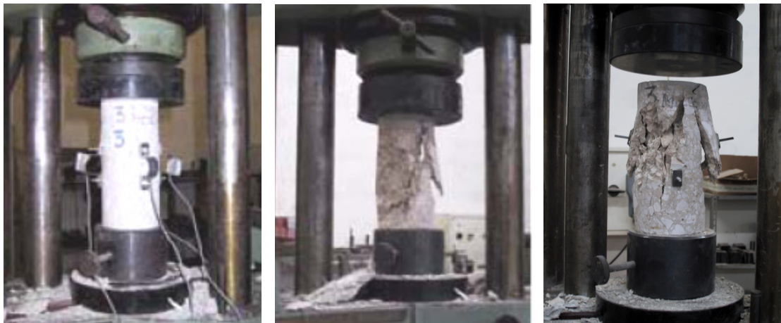
Figure 9. Compression Test on Concrete Cylindrical Specimen
