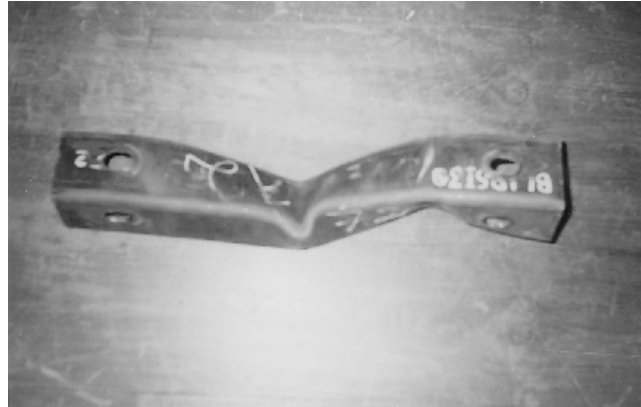
Figure 13. Failure of Single Angle by Local Plate Buckling under Bolted End Connection
