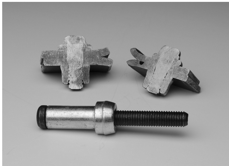
Figure 2. State of the Filling of Holes in Sheet Iron by Bolts
