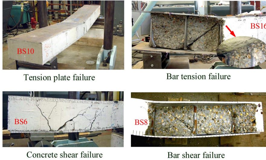
Figure 4. Typical Beam Static Failure Modes
