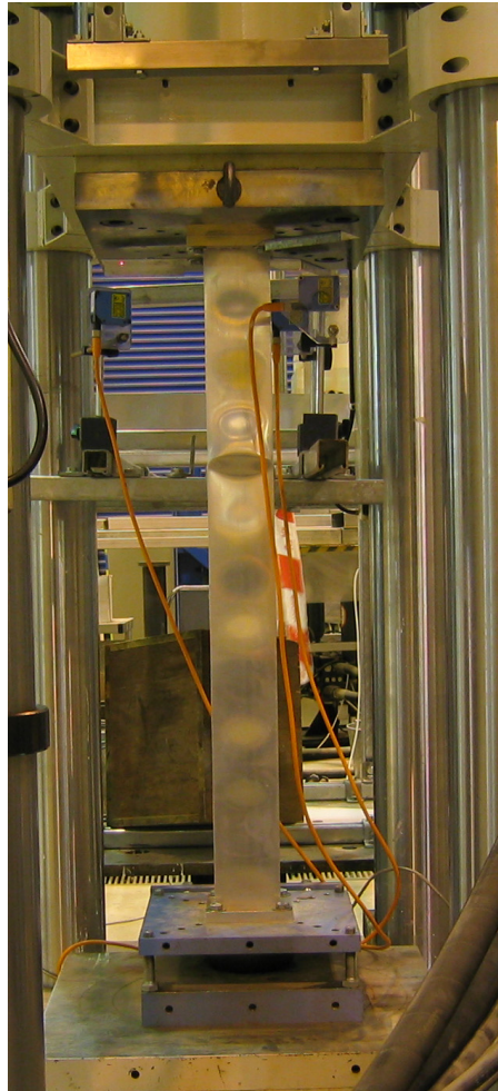
Figure 2. Column Specimen Failed by Local Buckling
