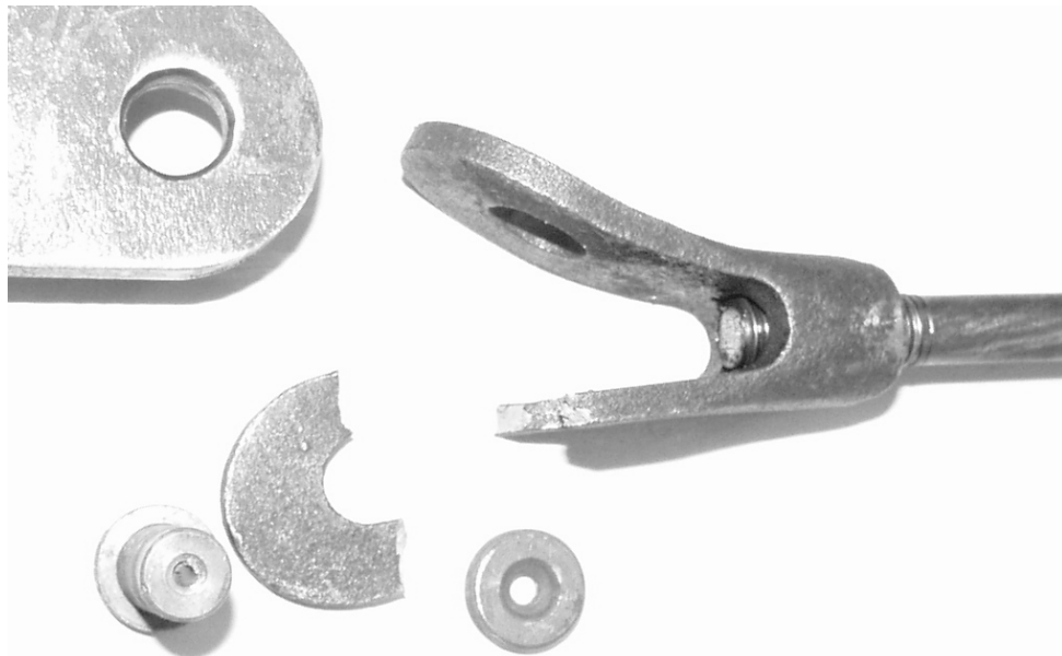
Figure 10. Broken Fork End Connector after Ultimate Load Test
