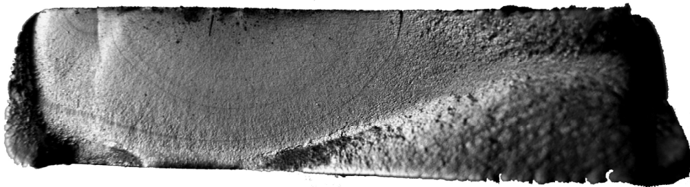
Figure 6. Cross Section of S1100 Specimen Showing Crack Marking Boundary Lines
