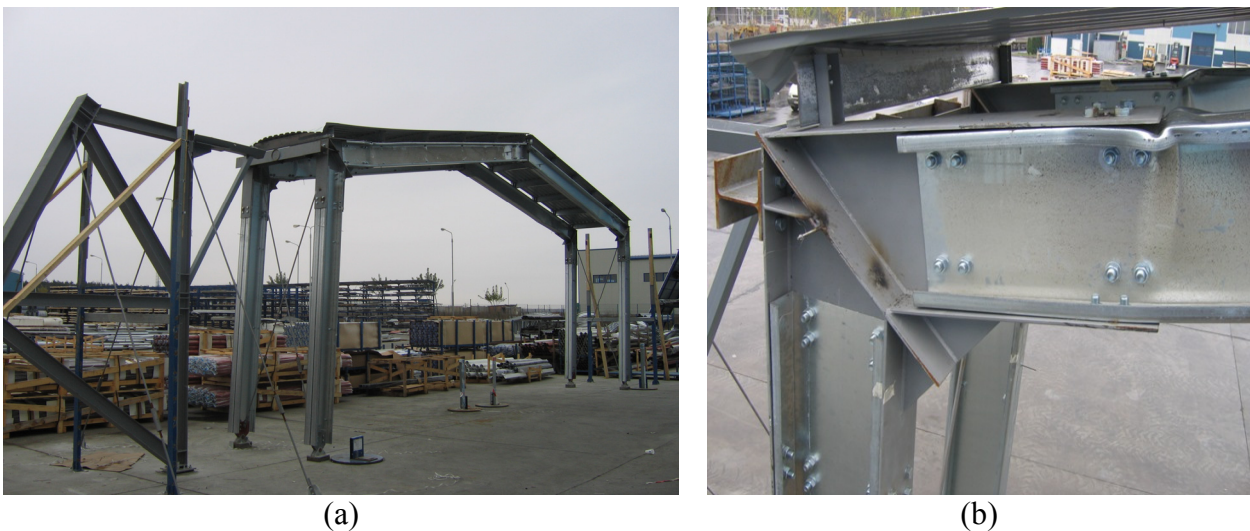
Figure 18. C1 Frame: Global View (a) and Local Buckling of the Left Beam Connection (b)
