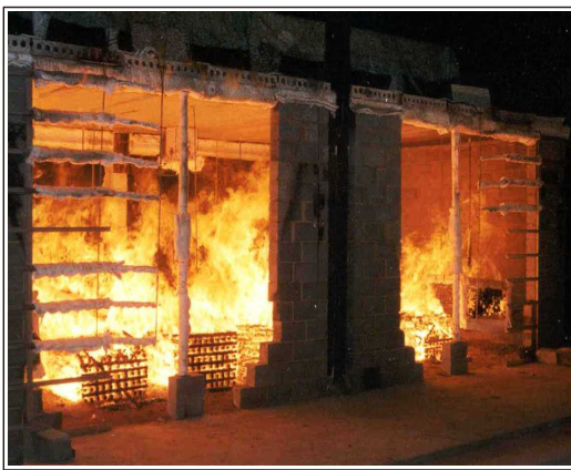
Figure 5. BRE Large Compartment Fire Test Figure 6. BRE Large Compartment Fire Modelling
