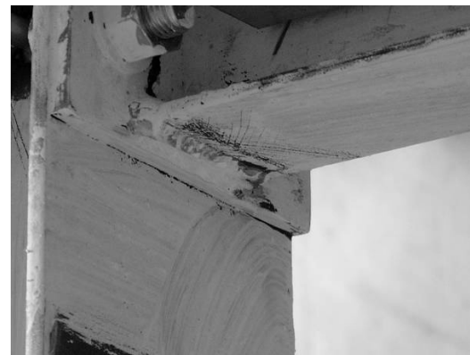
Figure 25. Yielding of Steel Components at the External Composite Joints
