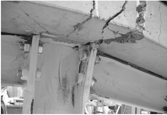
Figure 29. Spread of Yielding in the Steel Components of the External Composite Joints
