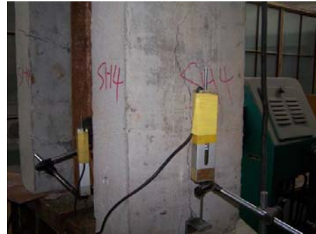
(a) The Transverse Cracks on the Side Profile (b) The Longitudinal Cracks on the Front Profile Figure 8. Lateral and Vertical Cracks of Push-out Specimens during the Test
