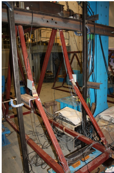
Figure 4. The Failure Shape of Steel Member Truss
