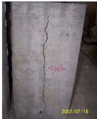
(a) Longitudinal Cracks on the Concrete Slab (b) Steel Component after the Removal of Concrete Figure 9. The Failure Conditions of Different Parts after Test
