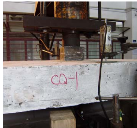
(b) Load Device of Local Compressive Test
