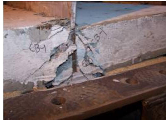
(b) Punch Failure of the Specimen
