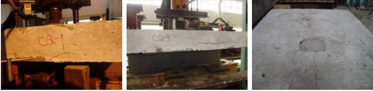
Figure 17. Phenomenon of the Local Compressive Test
