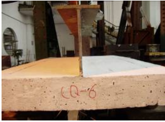
(a) Initial Cracks of the Specimen
