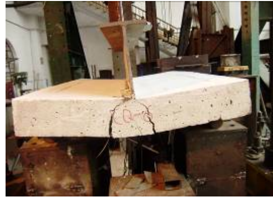
(b) Shear-bending Failure of the Specimen
