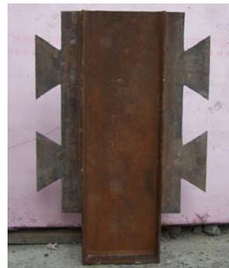
(a) Longitudinal Cracks on the Concrete Slab (b) Steel Component after the Removal of Concrete Figure 9. The Failure Conditions of Different Parts after Test
