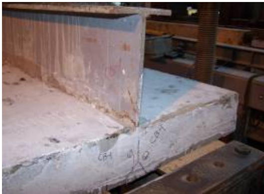
(a) Initial Cracks of the Specimen
