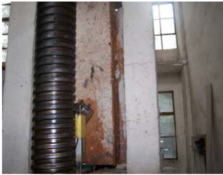
(a) The Transverse Cracks on the Side Profile (b) The Longitudinal Cracks on the Front Profile Figure 8. Lateral and Vertical Cracks of Push-out Specimens during the Test
