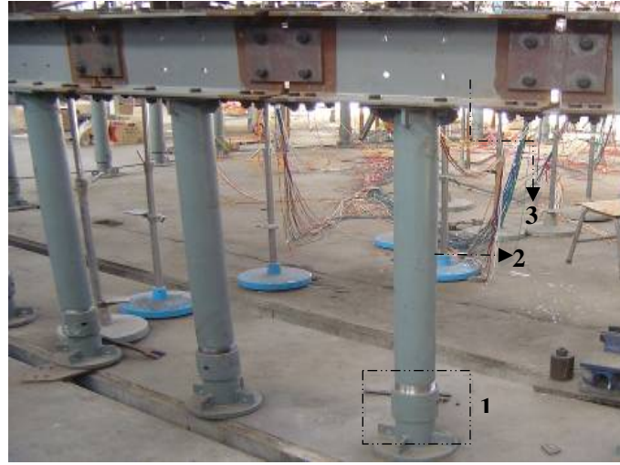
1-tunable socket 2-pillar 3-beam
