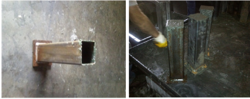
Figure 1. The Square Column Specimens before and after Concrete Filled
