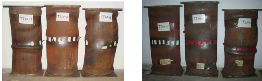
Figure 16. Behavior of the Specimens after Loading of the CFEST Short Columns
