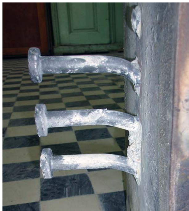
Figure 13. Deformed Shape of Headed Studs after Failure of LDA1 Specimen
