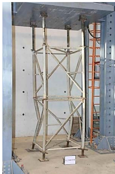
Figure 21. Failure Mode of Two-layer Setup with Extension of Top Screw Jacks
