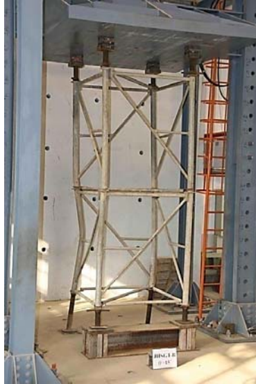
Figure 15. Failure Mode of Two-layer Setup with 33.2 cm Difference in Ground Elevation
