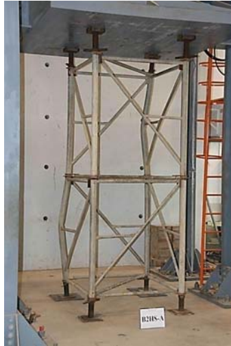
Figure 11. Failure Mode A of Two-layer Basic Setup in Test
