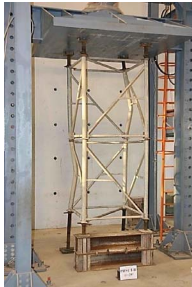
Figure 19. Failure Mode of Two-layer Setup with 56 cm Difference in Top Elevation
