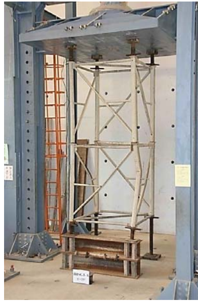
Figure 17. Failure Mode of Two-layer Setup with 56 cm Difference in Ground Elevation
