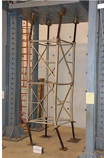
Figure 23. Failure Mode of Two-layer Setup with Extensions of Both Top and Base Screw Jacks
