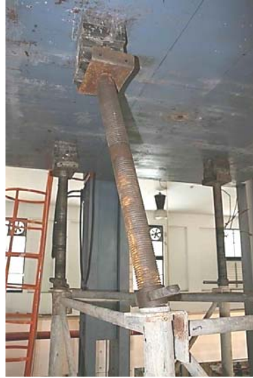
Figure 24. Failure at Connecting Joints between Top Screw Jacks and Vertical Members Observed in Test of Extension of Both Top and Base Screw Jacks
