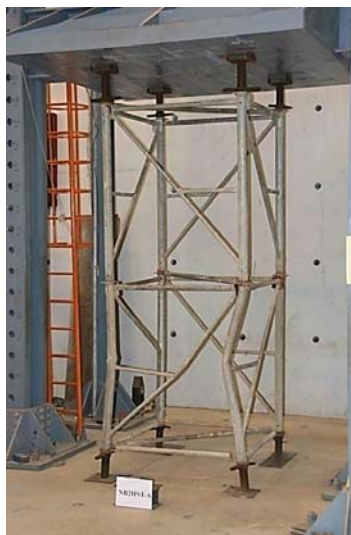
Figure 13. Failure Mode of Two-layer Setup with Non-stiffened Base Screw Jacks
