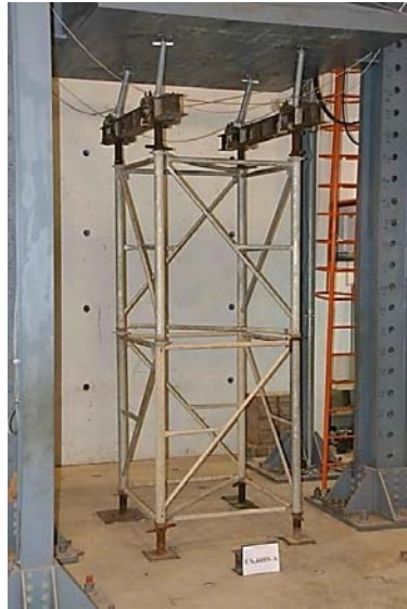
Figure 26. Failure Mode of Two-layer Setup Reinforced with Steel Tube Shores without Enclosed Restraint
