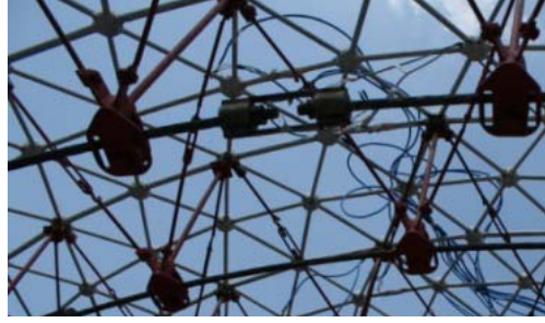
Figure 8. Device for Measuring Cable Force
