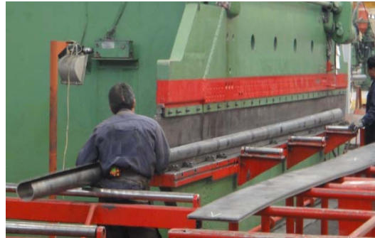
b) Bending of the plate with hydraulic press
