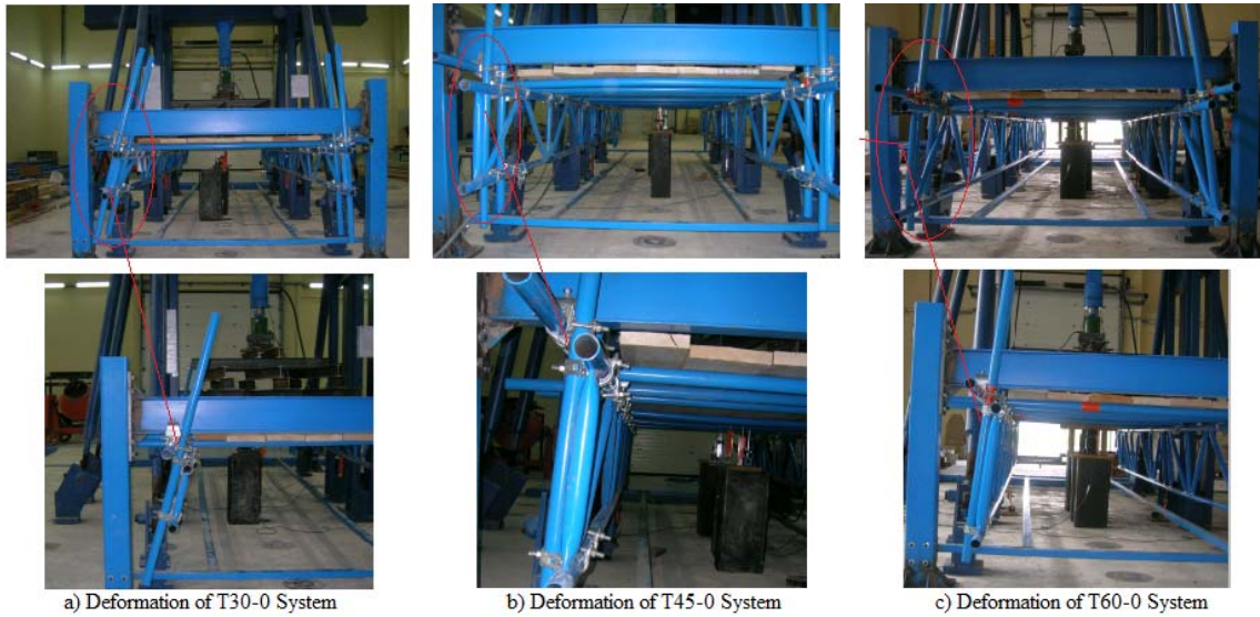
Figure 8. Deformation of some scaffolding systems during the loading tests
