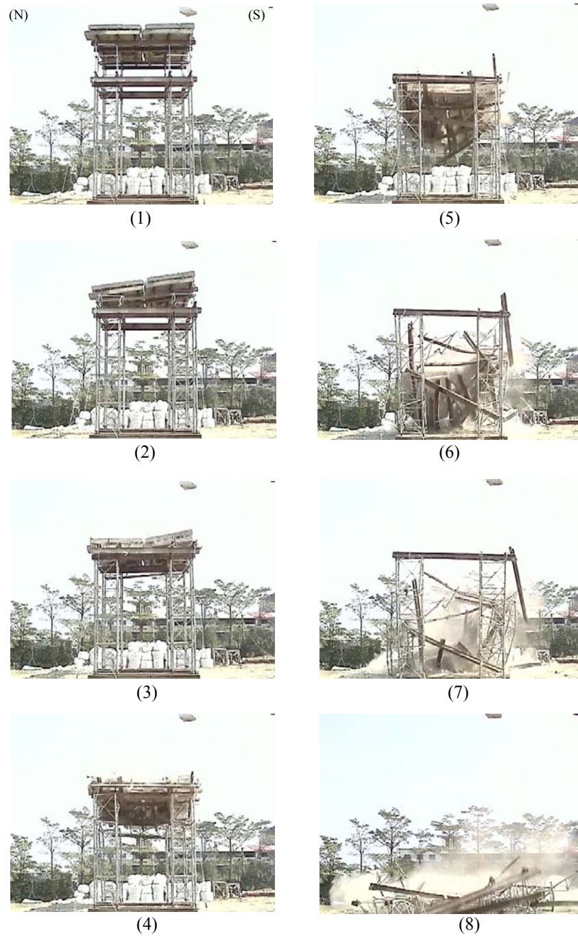
Figure 16B. Collapse of Outdoor Heavy-duty Scaffolds with Shores under Loading, as recorded by Camera on the West
