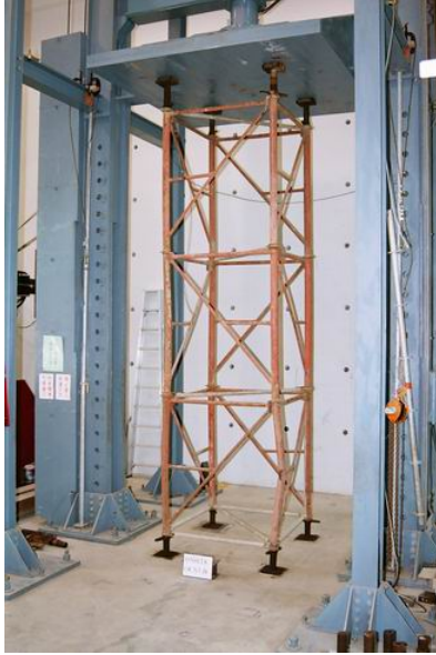
Figure 23. Failure Model for Three-story Reusable Independent Heavy-duty Scaffolds Treated with Red Lead Antirust Paint under Loading
