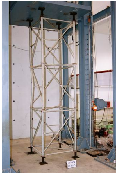
Figure 19. Failure Model for Three-story Independent Heavy-duty Scaffolds with Eccentric Load under Loading
