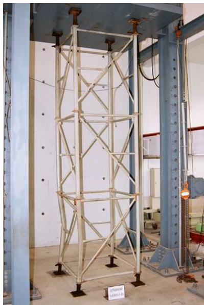
Figure 18. Failure Model for Three-story Independent Heavy-duty Scaffolds without Horizontal Braces under Loading
