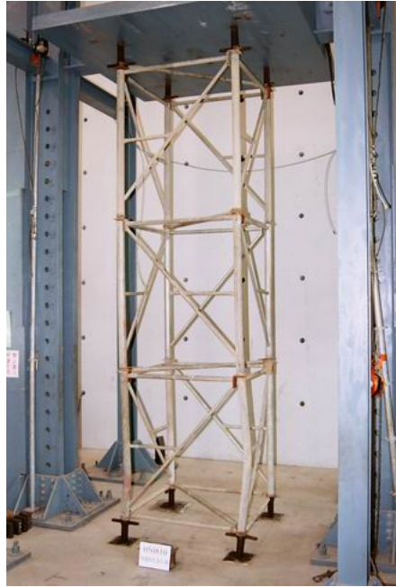
Figure 16. Failure Model for Three-story Independent Heavy-duty Scaffolds without End Plates of Top and Base Screw Jacks under Loading
