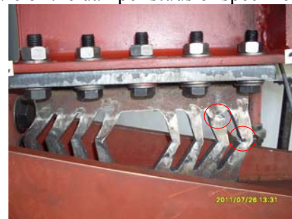
Failure of the damper studs of specimen 12D
