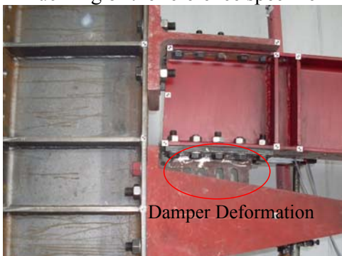
Damper deformation of specimen 15D
