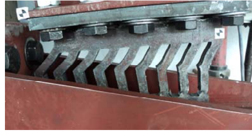
Failure of the damper studs of specimen 22E
