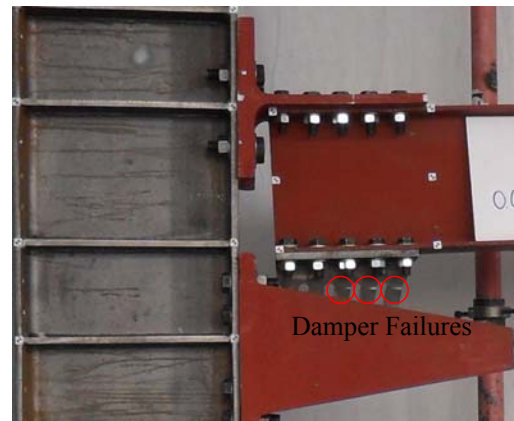
Failure of the damper studs of specimen 12D
