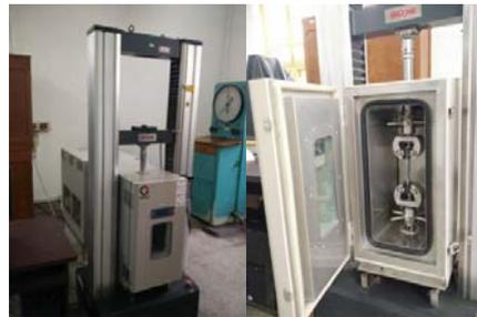
(a) The Tensile Testing Machine
