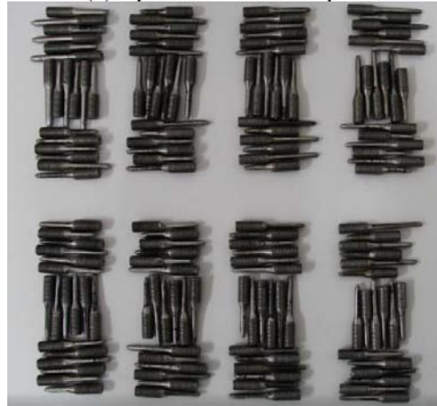
(b) Specimens after Tensile Test
