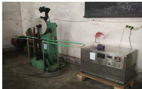
(b) The Pendulum Impact Testing Machine
