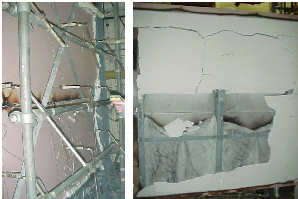
(a) Behaviour of gypsum plasterboard (before removal of plasterboard)
