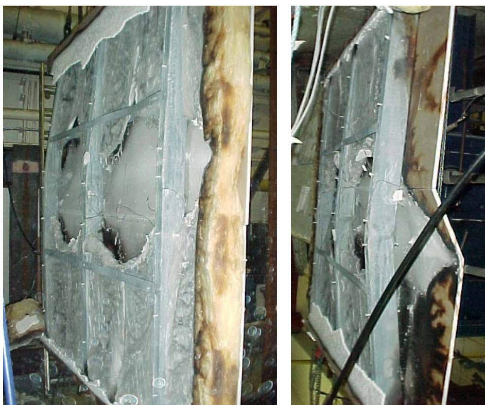
(a) Behaviour of gypsum plasterboard (before removal of plasterboard)
