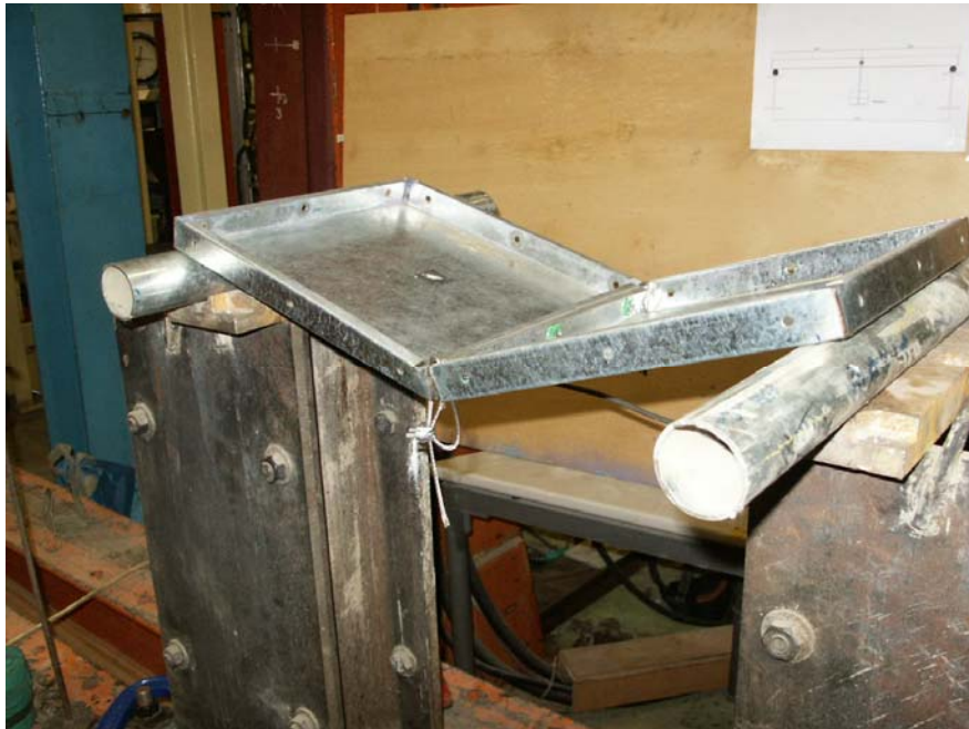
Figure 12. Failure mode of specimen BP1
