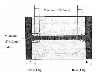
Figure 3. Clip Dimension Requirements
