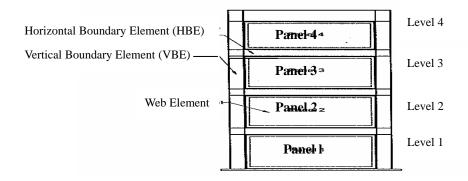
Figure 2. Schematic of Special Plate Shear Walls
