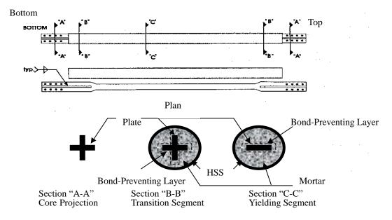
Figure 1. Details of a Buckling Restrained Brace
