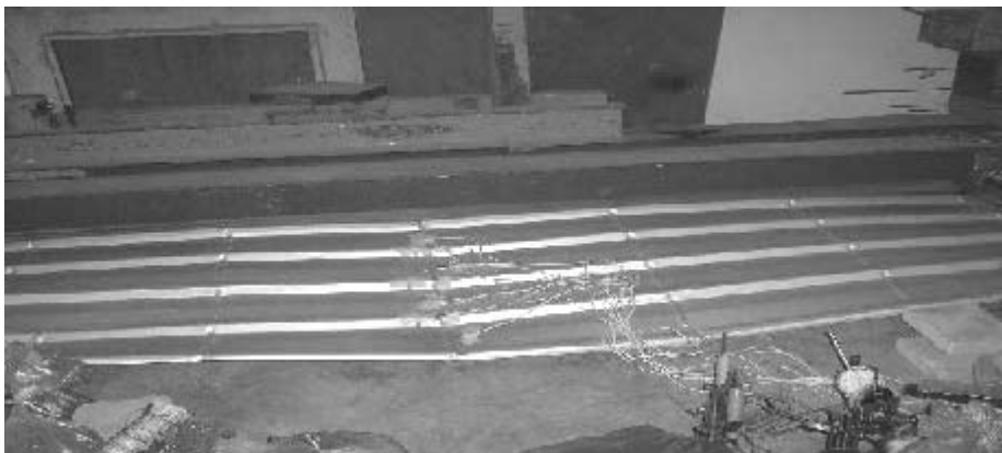
Figure 32. Experimental deflected shape of 0.25 m crown height parabolic roofing element
