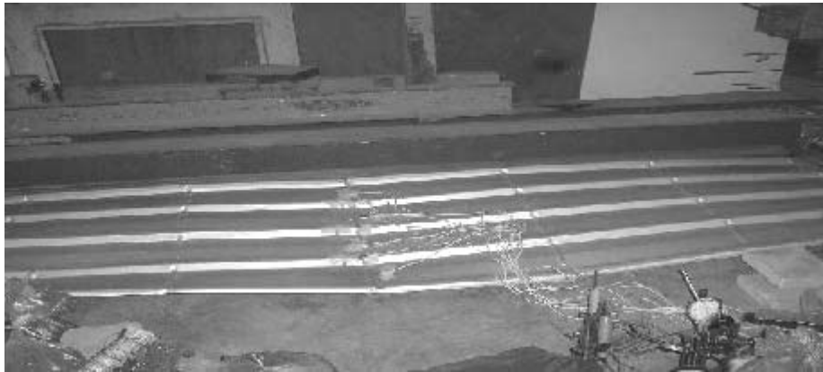
Figure 30. Experimental deflected shape of 0.125 m crown height parabolic roofing element
