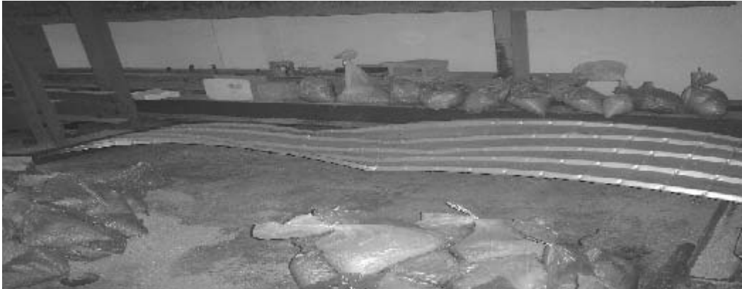
Figure 34. Experimental deflected shape of 0.5 m crown height parabolic roofing element
