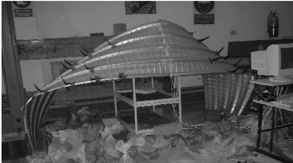
Figure 38. Experimental deflected shape of 1.5 m crown height cylindrical roofing element
