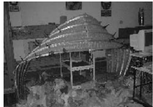
Figure 11. Experimental deflected shape of cylindrical roofing element
