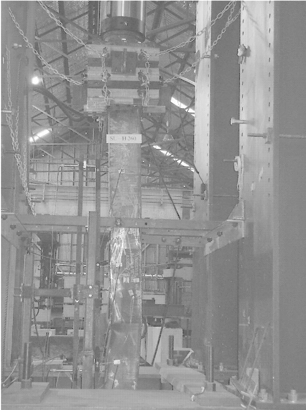
Figure 28. Failure Mode of Hollow Slender Column SL-H260
