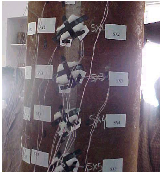
Figure 2. Marking of Strain-gauges
