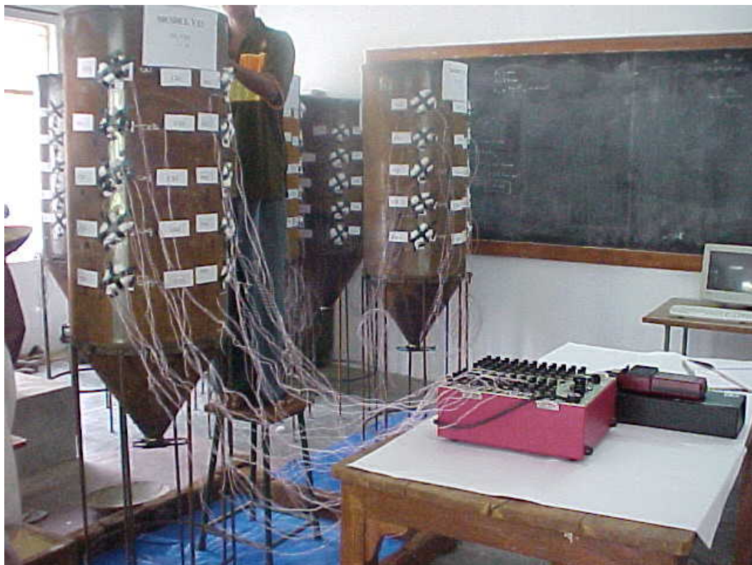
Figure 3. Silo Model Filled with Sand
