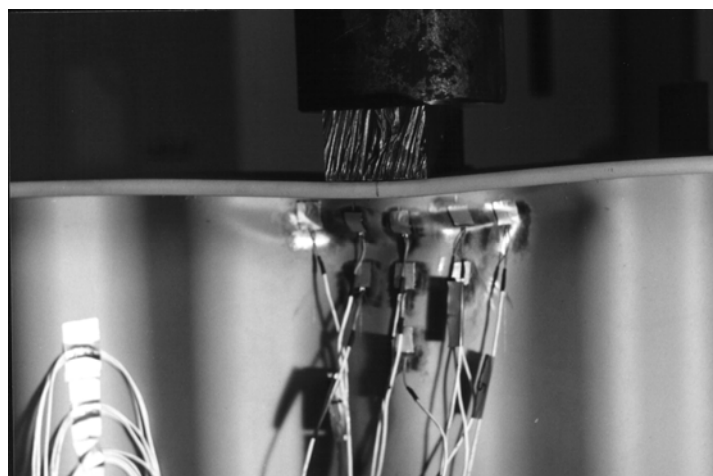
Figure 9 Form of Failure for Web and Flange of Girder "A"
