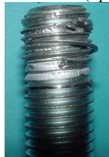
(b) Mode B: Bolt-thread Stripping (Specimen EEP_15_1, bolt #3)
