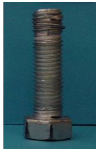
(b) Mode B: Bolt-thread Stripping (Specimen EEP_15_1, bolt #3)
