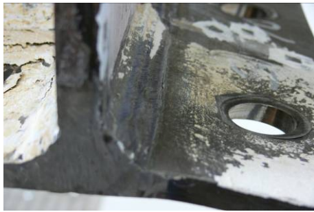
(a) Mode A: Cracking of the End Plate in the Heat Affected Zone (Specimen EEP_10_2(M27))
