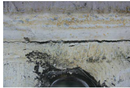
(a) Mode A: Cracking of the End Plate in the Heat Affected Zone (Specimen EEP_10_2(M27))
