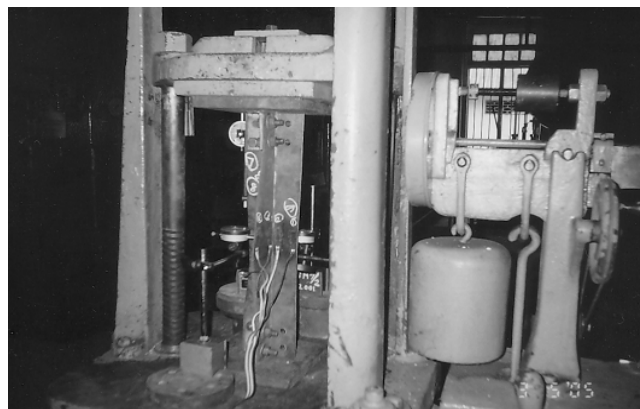
Figure 5. Test Set Up for Bolted End Connection
