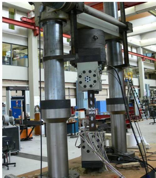
Figure 3. 600 kN Dynamic Servo Hydraulic Test rig of the Stevin Laboratory, TU Delft
