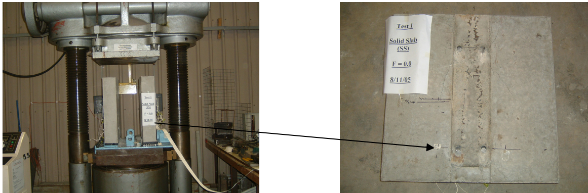
Figure 9. Concrete Damage at the Base of the Shear Connectors for Concrete with F=0 fibres
