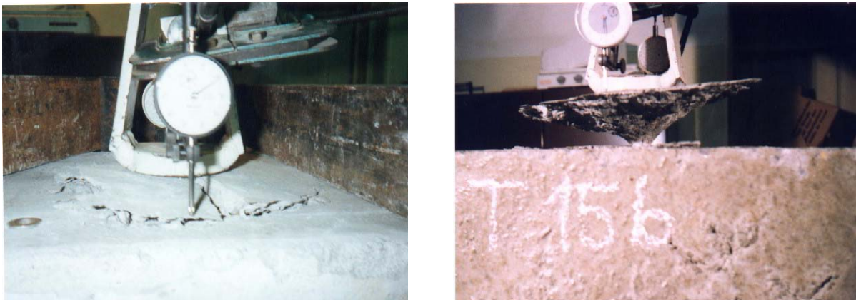
Figure 2. Illustration of Concrete-Cone Failure Mode: Tension Loading, Anchor in Large Edge Distance
