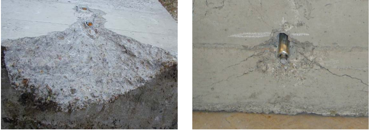
Figure 11. Illustration of Lateral Concrete-Cone Failure (Half Concrete Cone) Mode: Shear Loading, Anchor in Small Edge Distance
