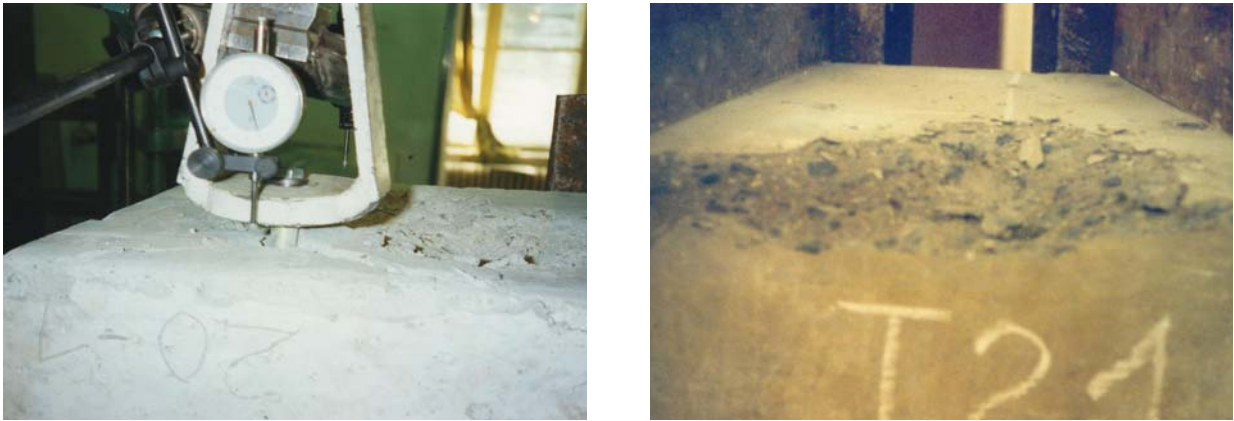
Figure 6. Illustration of Lateral Concrete-Cone Failure (Edge Failure) Mode: Tension Loading, Anchor in Small Edge Distance
