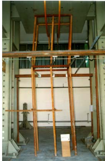
Figure 18. Test Results on Double-layer Shoring System with Horizontal Braces
