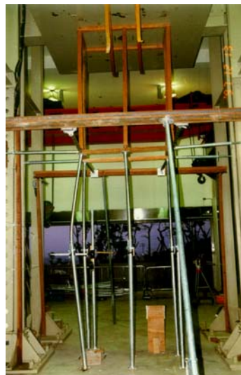
Figure 24. Test Results on Double-layer Shoring System with Combined Setup of Shores
