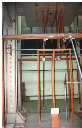
Figure 20. Test Results on Double-layer Shoring System with Axial Force Indirect Transfer
