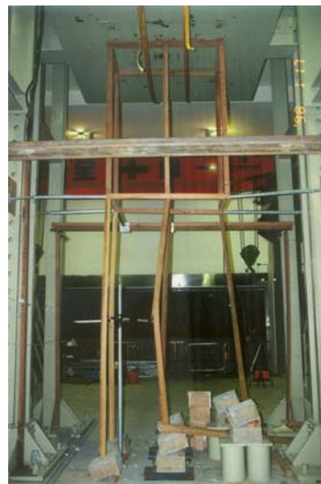
Figure 22. Test Results on Double-layer Shoring System with Inclined Boundary Condition
