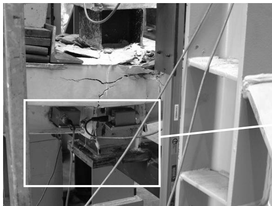
Figure 30. Deformation of the Internal Composite Joint at Point “D” of Figure 24
