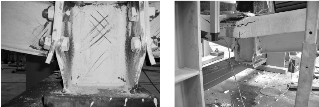
Figure 35. Internal Composite Joints at the End of the Test
