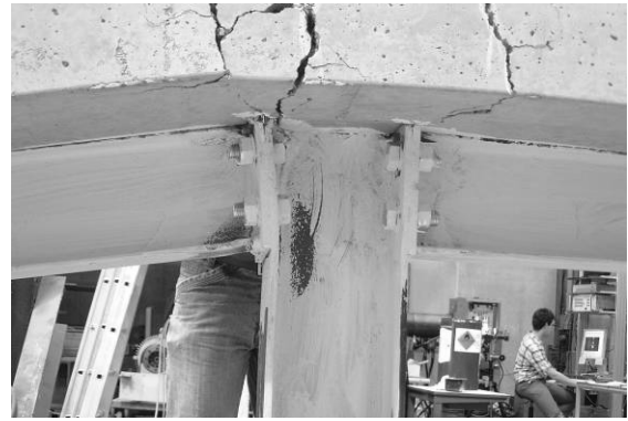
Figure 29. Spread of Yielding in the Steel Components of the External Composite Joints
