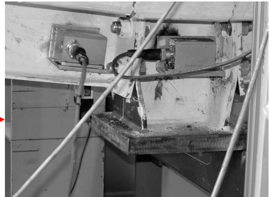
Figure 30. Deformation of the Internal Composite Joint at Point “D” of Figure 24
