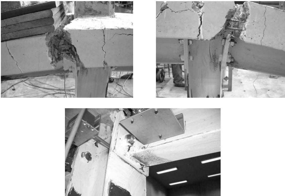
Figure 34. External Composite Joints at the End of the Test
