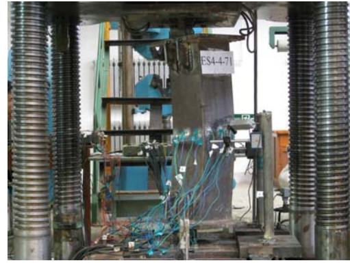
Figure 4. The Typical CFST Column Specimen after Testing
