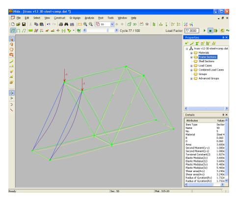
Figure 8. The Analytical Model of the Truss
