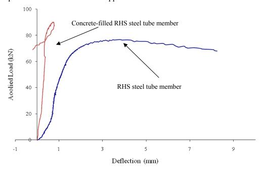
Figure 6. Load against Out-of-plane Deflection of Failure Member
