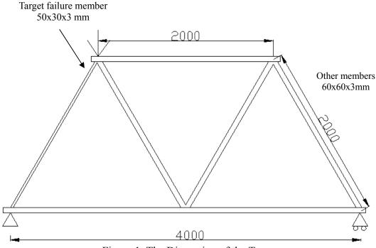
Figure 1. The Dimension of the Trusses
