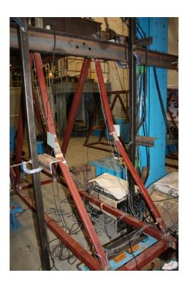
Figure 4. The Failure Shape of Steel Member Truss
