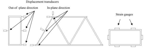
Figure 2. Displacement Transducers and Strain Gauges Location
