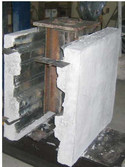
Figure 1. A Photo of a Specimen Prepared for the Push-out Tests [12]
