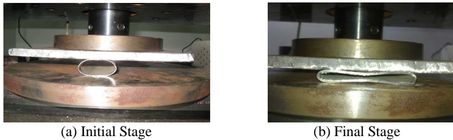
Figure 6. Static Compression Experiment of Single Circular Steel Tube
