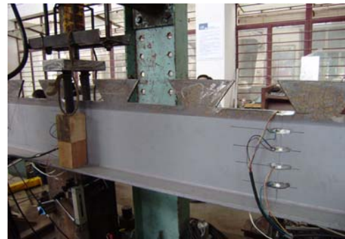
(a) Loading at One Side of the Steel Beam Web (b) Loading at Both Side of the Steel Beam Web
