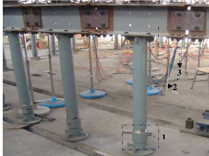
1-tunable socket 2-pillar 3-beam
