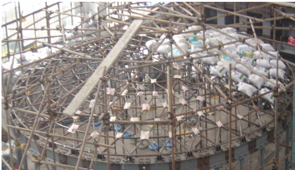
Figure 13. Loading of Heap Load
