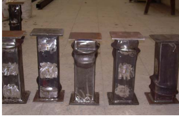
Figure 7. Typical Specimen Failure Modes
