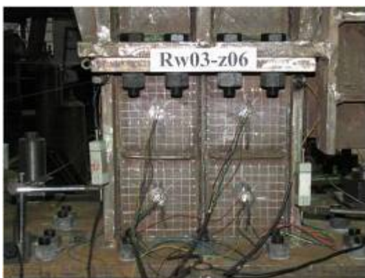
Figure 3. Stiffened Shear Panel Dampers
