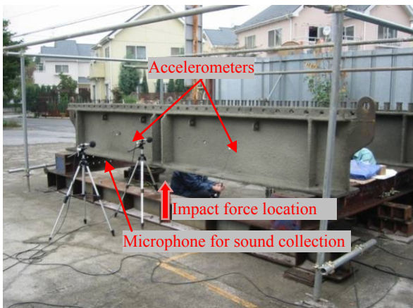
Figure 21. Set-Up of the Impact Test
