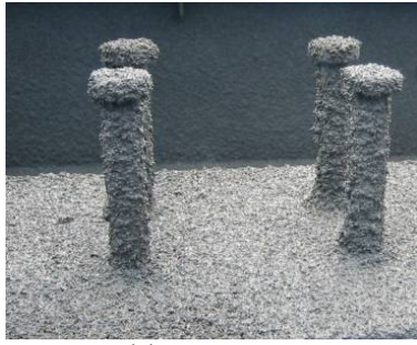
Figure 27. Rubber-Latex Mortar on Studs
