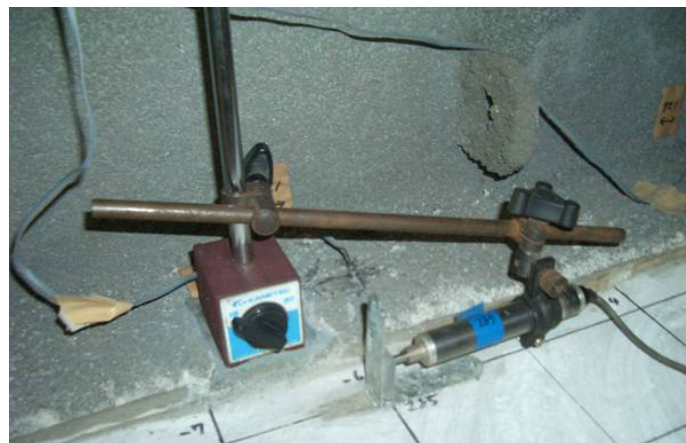
Figure 23. Arrangement of the Linear Variable Differential Transducers (LVDTs)
