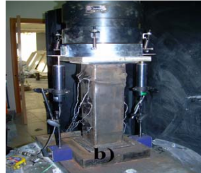
3b. The Test Setup for the Square Columns
