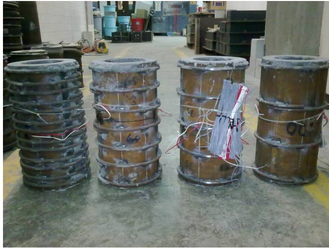
Figure 1(b) Double-skinned NSCFST columns with external steel rings ( s=5t_o , 10t_o , 15t_o and 20t_o ) with Hollow Ratio of 0.72
