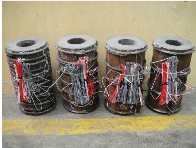
Figure 1(e) Double-skinned HSCFST columns with external steel rings ( s=5t_o , 10t_o , 15t_o and 20t_o ) with hollow ratio of 0.56
