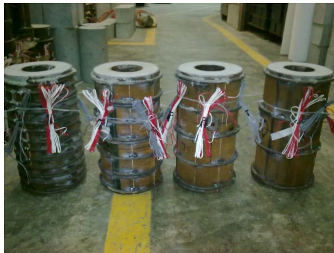
Figure 1(a) Double-skinned NSCFST columns with external steel rings ( s=5t_o , 10t_o , 15t_o and 20t_o ) with Hollow Ratio of 0.56
