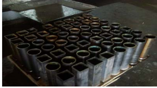
Figure 1. The Square and Circular Column Specimens before Concrete Filled
