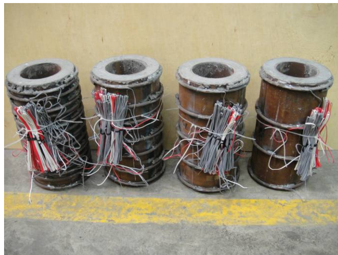
Figure 1(f) Double-skinned HSCFST columns with external steel rings ( s=5t_o , 10t_o , 15t_o and 20t_o ) with hollow ratio of 0.72
