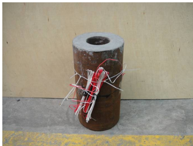
Figure 1(g) Double-skinned HSCFST columns without external steel ring with hollow ratio of 0.56
