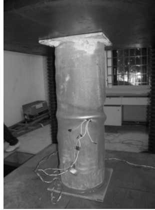
Figure 4. Load Bearing Capacity Experiment of the CFST Column
