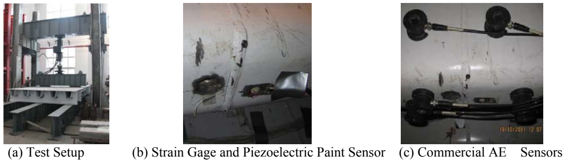
Figure 7. Laboratory Test Set-up and AE Sensor Placement
