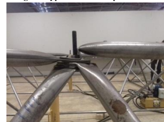
Fig. 38 Typical node collapse LT-02
