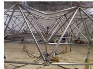
Fig. 47 Buckling of the top cords for LTDS prototypes
