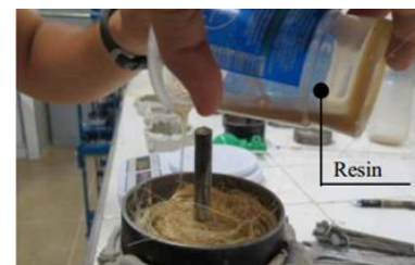
Fig. 23 Steel mold for make as space with PRSF
