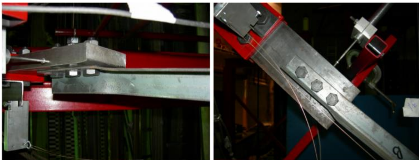
Fig. 12 Local failure of test specimens (2 and 3) [24]
