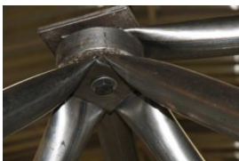
Fig. 43 No local collapse of node at chord buckling for LTDA-02
