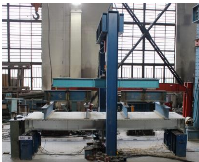
Fig. 4 Test setup of floor specimens
