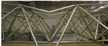
Fig. 42 Detail of buckled chord for LTDA-02
