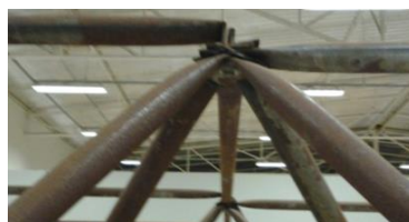
Fig. 20 Collapse in typical node (24kN) [1]
