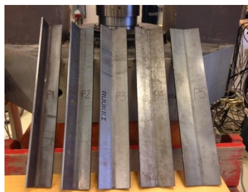
Fig. 1 L section profiles with different cold-formed angles
