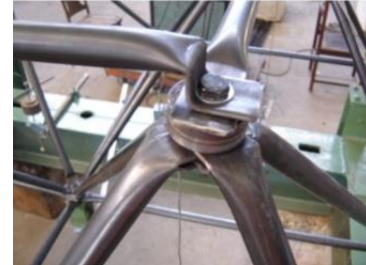
Fig. 15 Collapse of LTDE (38kN) [14]
