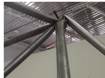
Fig. 37 Typical node collapse LT-01
