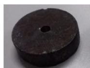
Figure (c)- Steel spacer: F_y = 250 MPa and \phi 75mm
