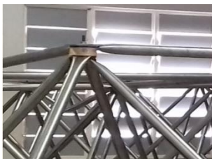
Fig. 48 Node after collapsing the Structure
