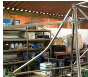
Fig. 16 Collapse of LTDME (P1 - 39kN)
