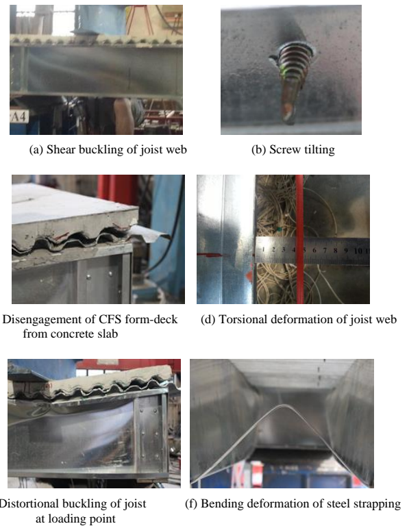
Fig. 5 Failure characteristics of BM-1
