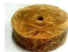
Fig. 25 Spacer made with sisal and resin PRSF [15].
