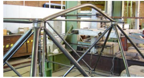
Fig. 14 Collapse for prototypes with LTDCE (42kN) [1].
