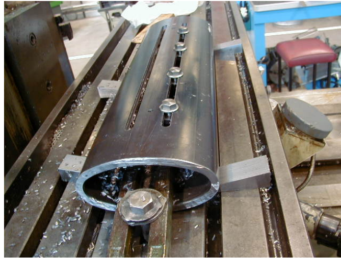
Figure 3. Machining of tensile coupons
