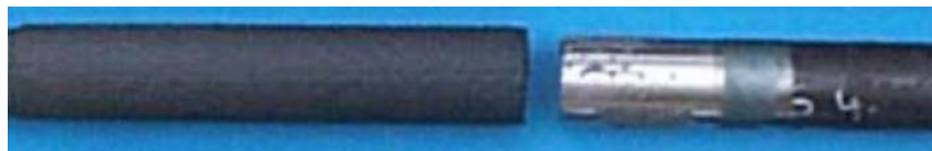
(c) Steel tubes with normal modulus CFRP (Jiao and Zhao (2004))
